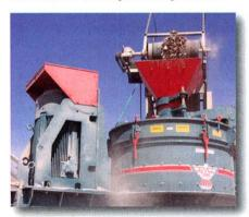
pabilities up to 400. A compact yet powerful option, this model weighs in at 19,000-lb. and is able to consistently produce up to 275 tph.
