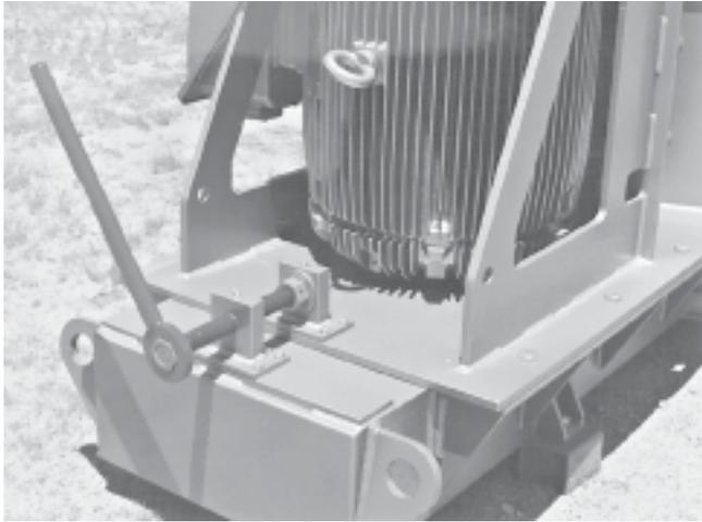
*Loosening the belt tension adjustment screw*
