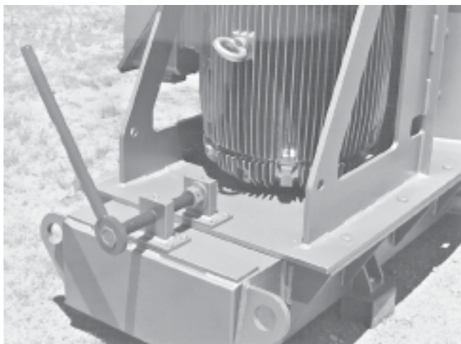
Loosening the belt tension adjustment screw
