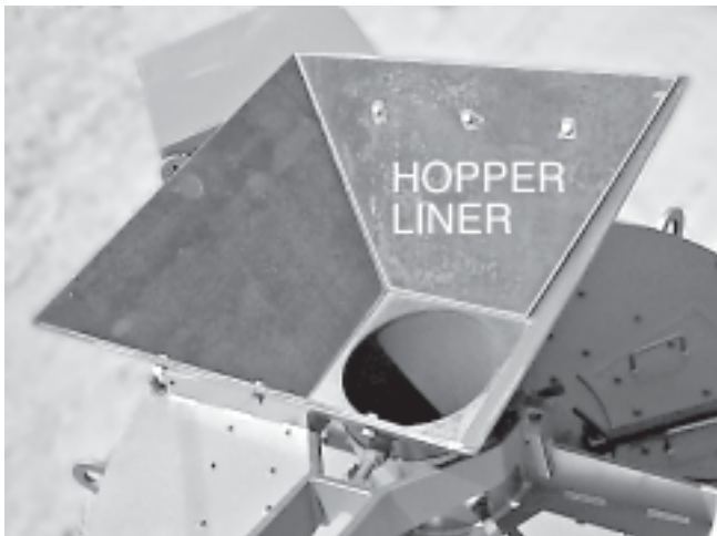
Feed hopper liner
