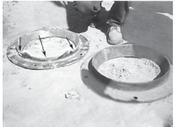
The feed tube liner above caused excessive tube flange wear. This tube flange lasted only 16 hours.
