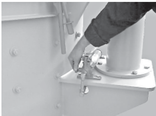
Relieving ram pump pressure
