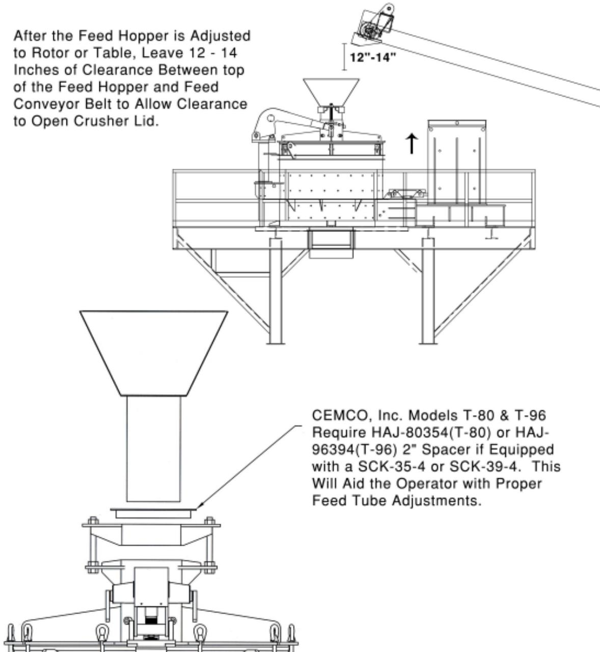
CEMCO, Inc. Models T-80 & T-96 Require HAJ-80354(T-80) or HAJ-96394(T-96) 2" Spacer if Equipped with a SCK-35-4 or SCK-39-4. This Will Aid the Operator with Proper Feed Tube Adjustments.
