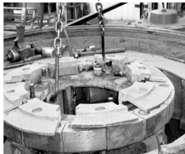
*Eyebolts attached to the rotor on opposite sides makes the rotor easy to lift with a crane.*
